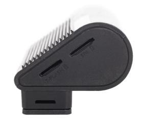
Attach the bracket of the front camera to the windshield. It is recommended to install it behind the rearview mirror to preserve a maximum field of vision when driving
